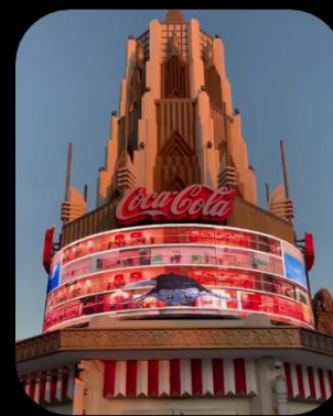
Minimum radius R \geq 0.6\text{ m} arc or cylinder
